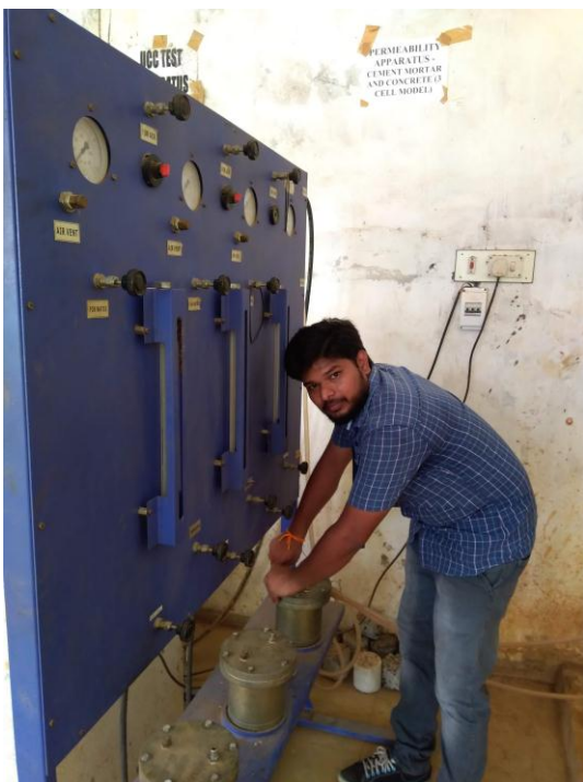
Fig: Permeability test working on lab
