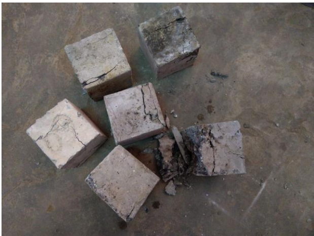
Fig: After testing on the compressive test on moulds
