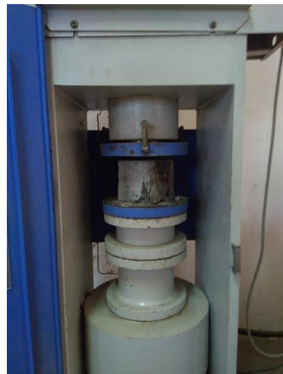
Fig: Compressive test on cubes
