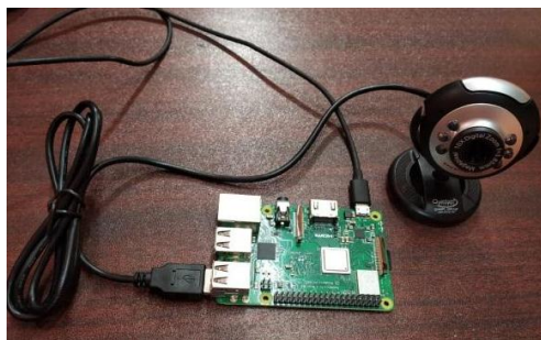
Fig -7: Stimulation using raspberry pi(face recognition and TTS)
