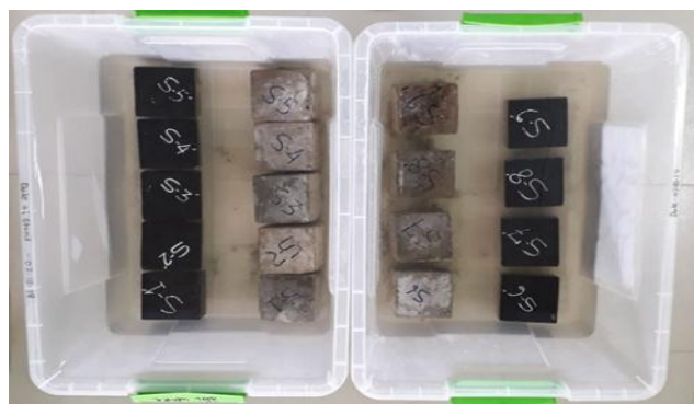
Figure 1: Durability test of concrete with or without protective surface coating of coal tar epoxy paint on concrete surface exposed to 4% Na 2 SO 4 solution
