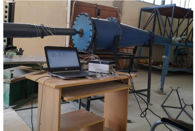
Fig 2.2.2: Supersonic wind tunnel facility with diffuser
