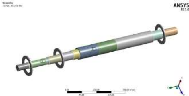
Figure -5.1: Final geometrical model used for modal analysis
