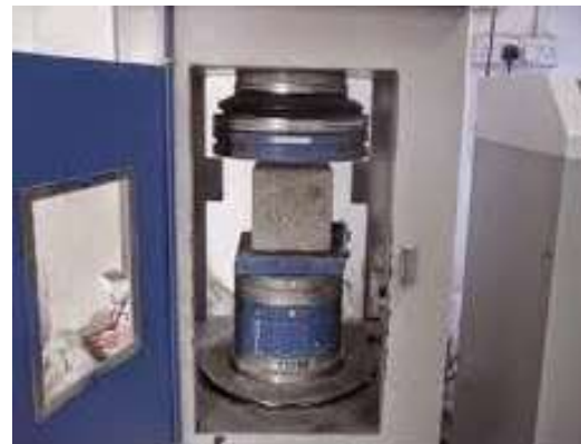
Fig.3 Compressive Strength test on cube
