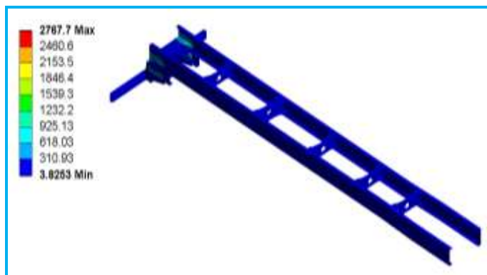
Fig-6: Temperature obtained from transient thermal analysis for weld path I is 2731.8 0C
