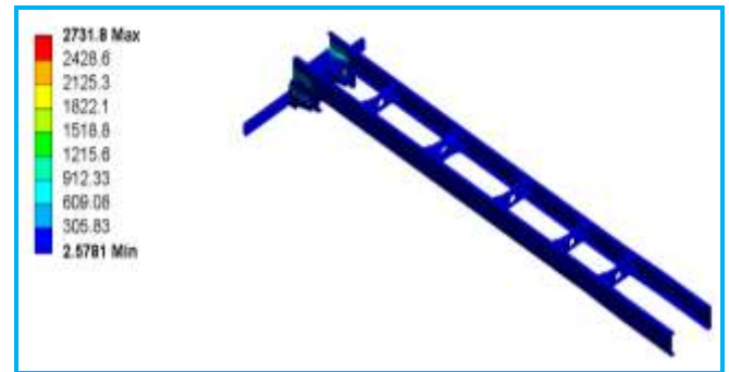
Fig-8: Temperature obtained from transient thermal analysis for weld path II is 2747.8 0C.
