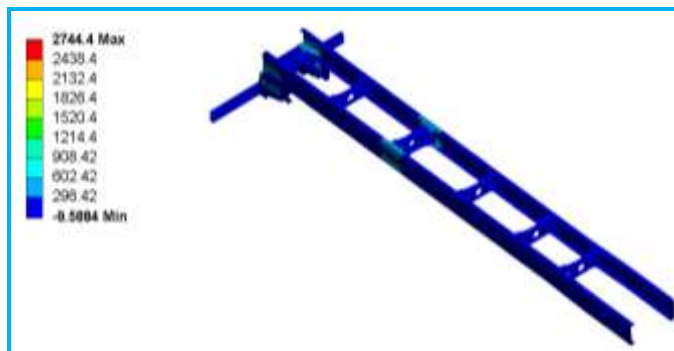
Fig-12: Temperature obtained from transient thermal analysis for weld path IV is 2744.4 0C
