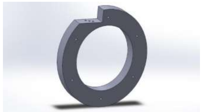
Fig -4: 3-D model of casing with L-shaped cut section.
