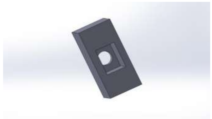
Fig -3: 3-D model of inlet chamber with fluid inlet at center.
