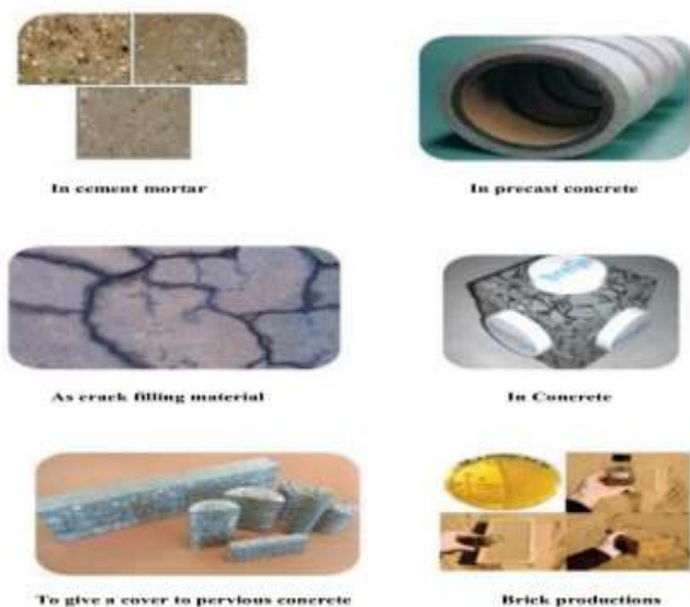
FIG 4: Application of Bacterial Concrete in Construction Area
