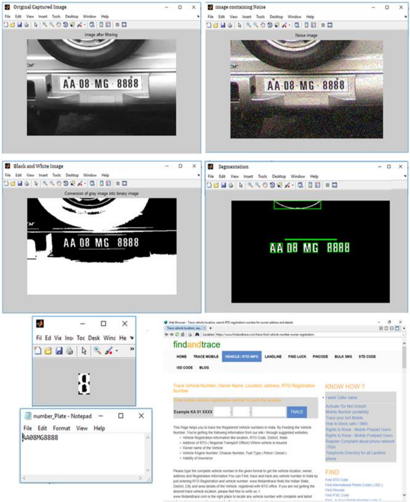
Fig -4: Operation of ANPR using MATLAB
