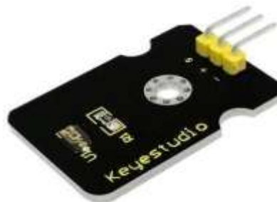
Fig -4: (TEMT 6000) Light Intensity monitoring sensor.
