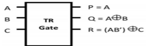
Fig -5: Block Diagram of TRG
