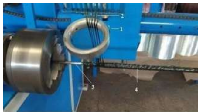
1 - Carriage, 2- Preimpregnated carbon fiber, 3-Mandrel, 4 - Carbon fiber winding on mandrel
