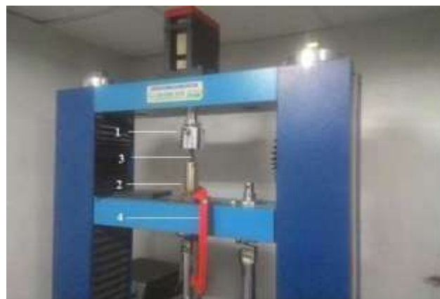
1- Upper fixture, 2- bottom fixture, 3- Carbon/Epoxy Rod, 4- Clamp
