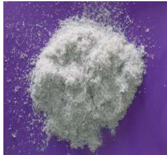
Pulverised Plastic material used in concrete
