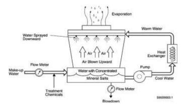
Figure 1: Function of cooling tower
