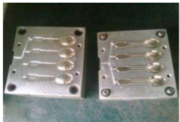
Fig. 2: Photograph of Old Dies Showing Core and Cavity
