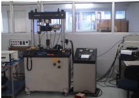
Figure: (3) Tensile test and Bending test of Laminate composites:
