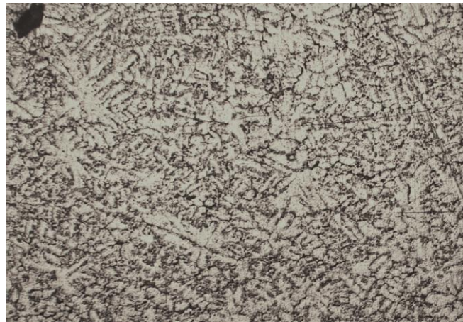
Fig. 2 Microstructure of A6082/SiC MMC
