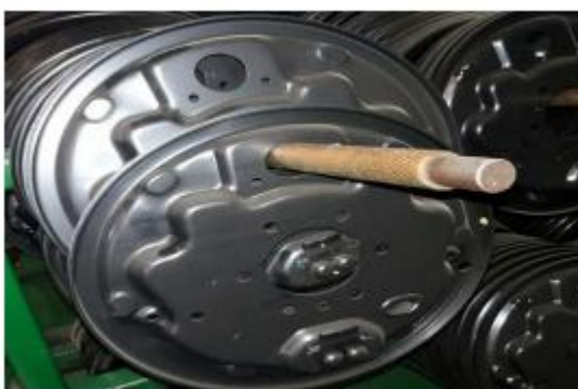
Figure-11. Dent due to bare trolley arm
