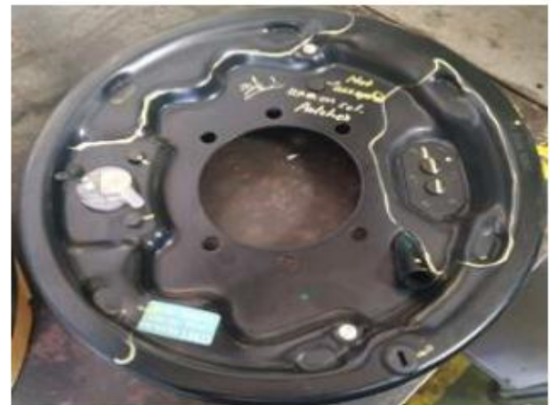
Figure-8. Defects of back plate
