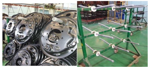
Figure-12. Trolley arms covered by plastic covers
