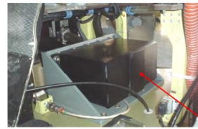
Figure 3.1.: Erahm Damper Installed in The Nose Area in Y Direction
