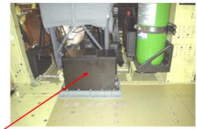
Figure 3.2.: Erahm Damper Installed in The Cabin (Behind Co Pilot Seat) in Z Direction
