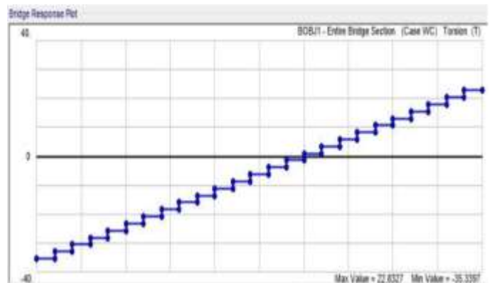
FIG -13: Torsion due to Wearing coat
