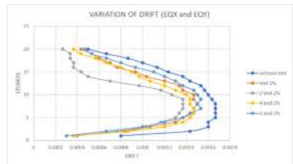
Fig. 9 (b) Comparing Drifts with Single and Multiple TMD of mass ratio 2% along EQX &EQY
