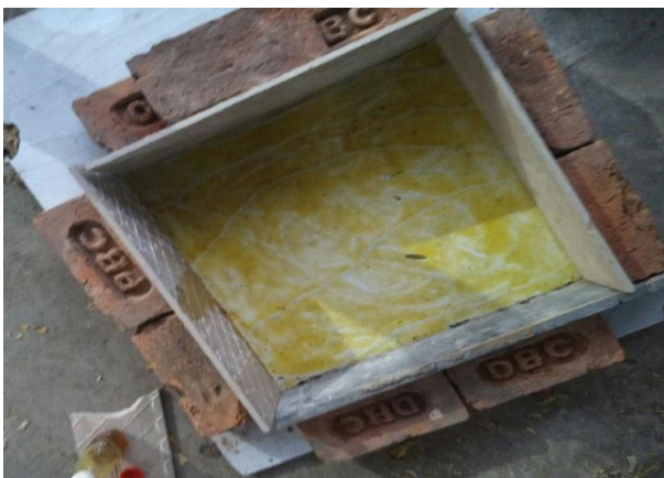
Fig. 10: Oiling Of Mold
