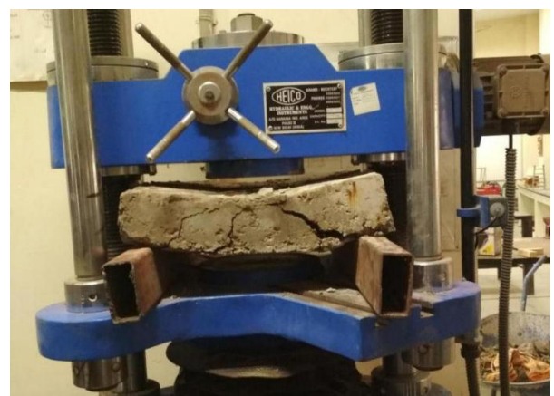
Fig. 17: Crack Formations after Loading
