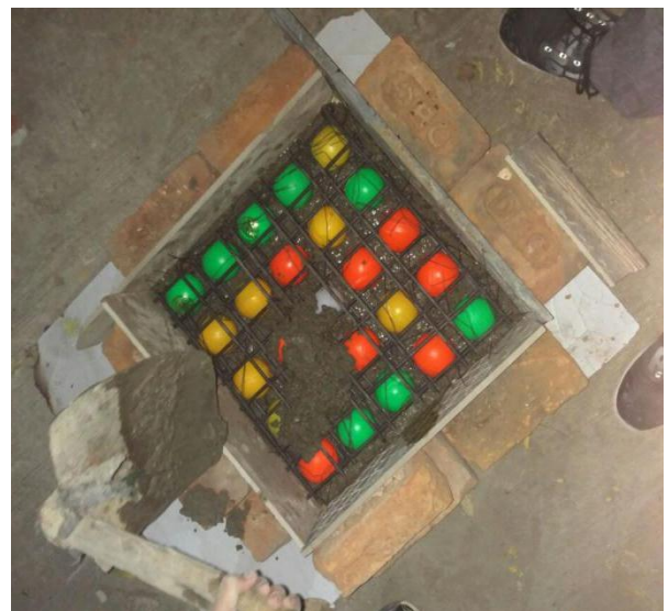
Fig. 12: Mixture Filling In Mould
