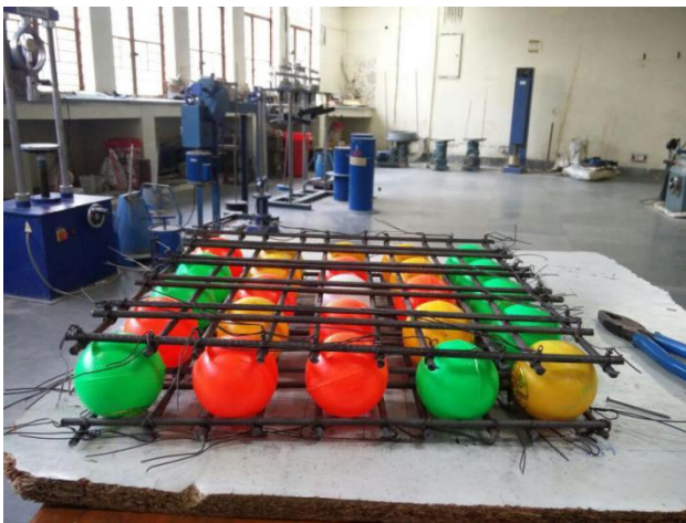
Fig. 9: Complete Mesh consisting Balls and Wires
