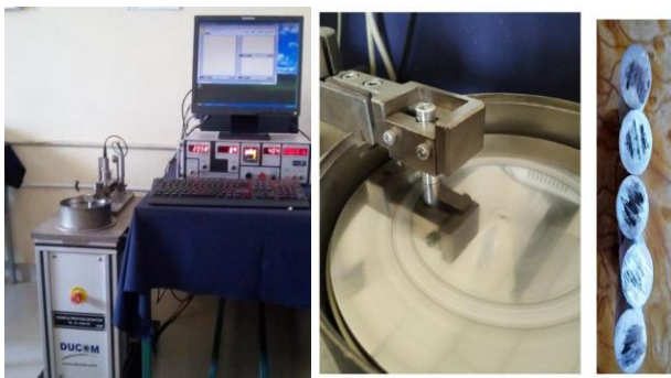
Figure 5: Wear testing set up and wear specimens after test
