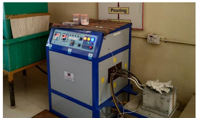
Figure 2: Stir casting set up
