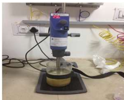
Fig. 2.1 Homogenizer used for mixing of nanoclay
