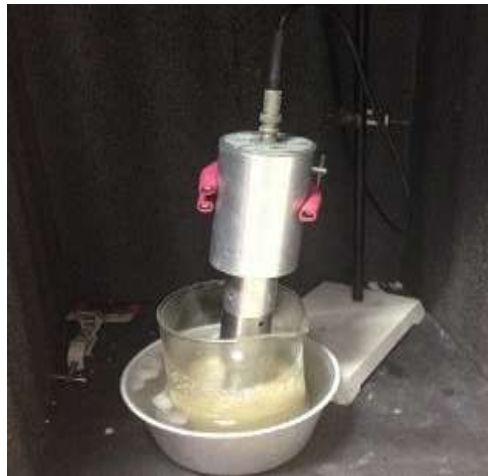
Fig. 2.2 Dispersion of nanoclay into epoxy resin with probe
