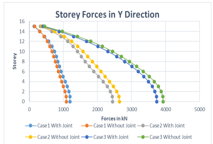
Graph 4.3: Storey Forces in kN of all three cases with and without Expansion Joint in X and Y Direction
