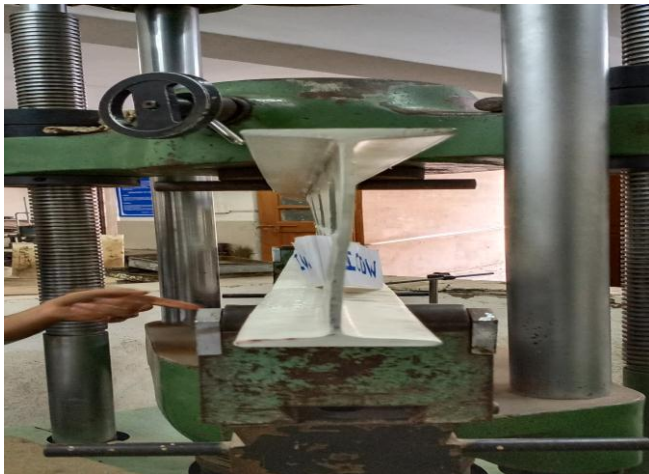
Fig -10: Showing Lateral torsional buckling of Web for ICSW 225
