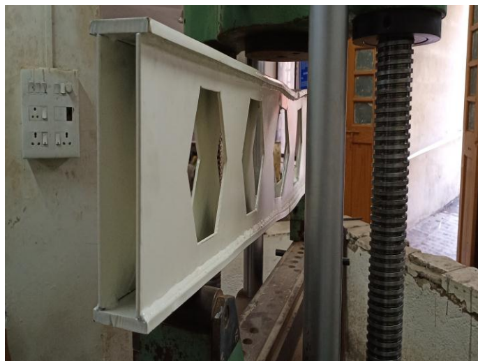
Fig -11: Showing Failure of compression flange for ICDW 225
