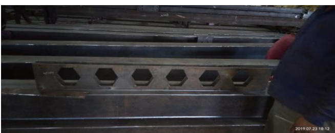
Fig -6: Fabrication of IC 225 for Single and Double web of Castellated beam
