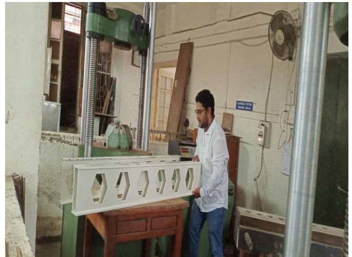
Fig -7: Single and Double Web Castellated beam
