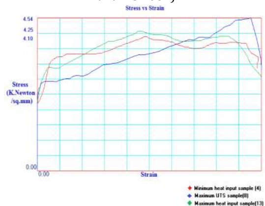
Figure 3. Stress strain curve for minimum heat input, maximum heat input and highest UTS sample
