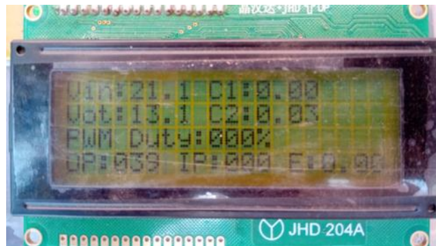
Fig. 15 LCD readings of No load operation
