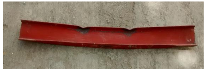
Fig 2: Before and after testing un-stiffened beam
