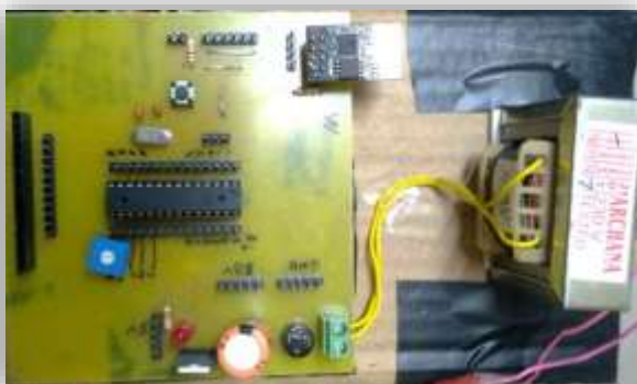
Figure 4.5:- Micro-controller IC circuit
