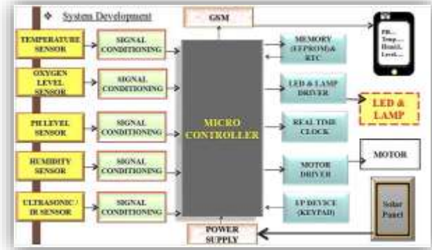
Figure 4.1:- System Block Diagram
