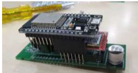
Fig -19: Hardware v4.0 IoT device (assembled)
