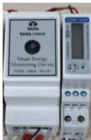
Fig -18: IoT device with a Single-Phase Meter
