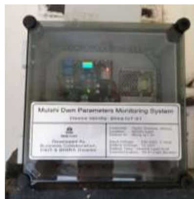
Fig -22: IoT device for Use Case 2 inside weatherproof IP68 enclosure
