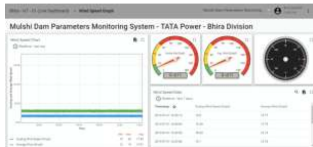
Fig -17: Dashboard board showing all historical and live wind related data from an Asset Monitoring Device
