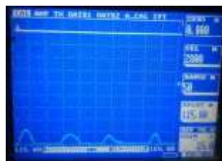
(b): Delaminated zone
