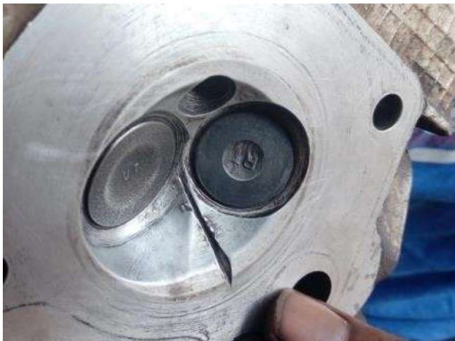
Fig. (2) Actual Grooved Engine Cylinder Head
