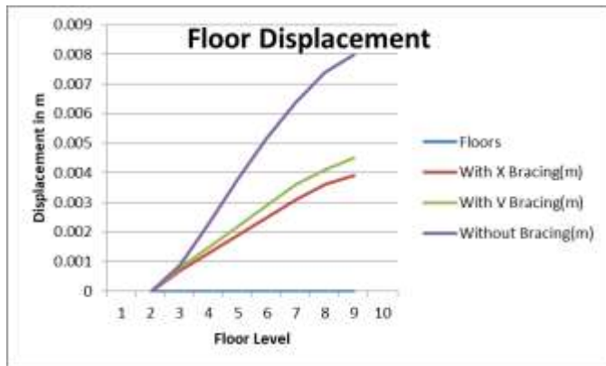
Figure: 3.1 Storey displacement of the model in X direction
