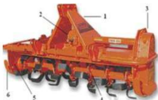
Fig-1: Rotavator and its main elements
