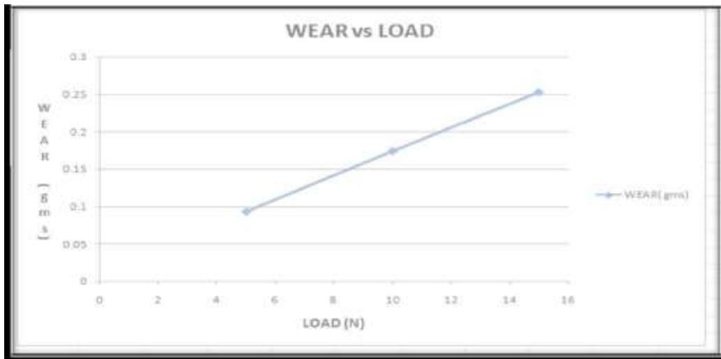
Curve 5: Variation of wear rate of the work piece for 150 rpm angular speed
