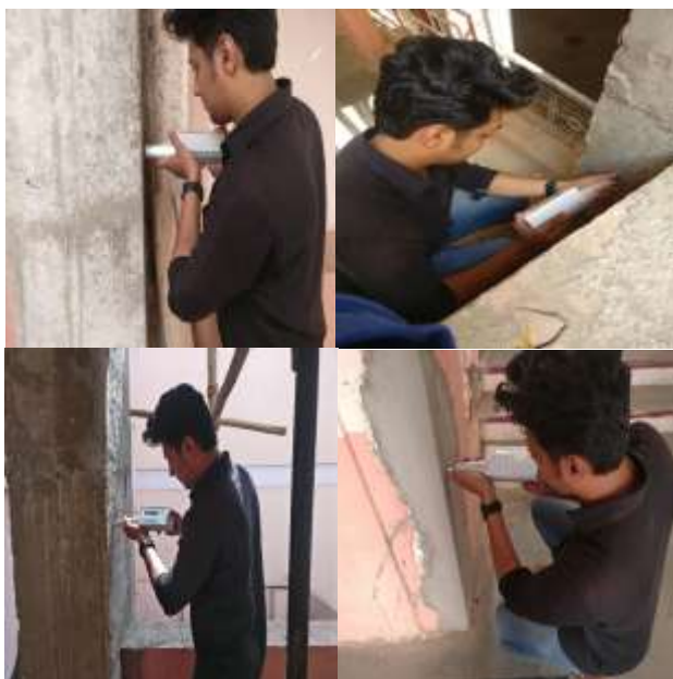
Fig-5: Rebound Hammer Test
