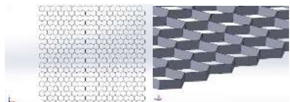
Image 1: The in-plane and out-of-plane directions of a honeycomb which are X and Y, and Z respectively.
