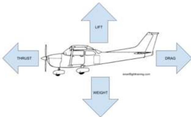
Fig -1: Four Forces acting on an aircraft/Drone's
