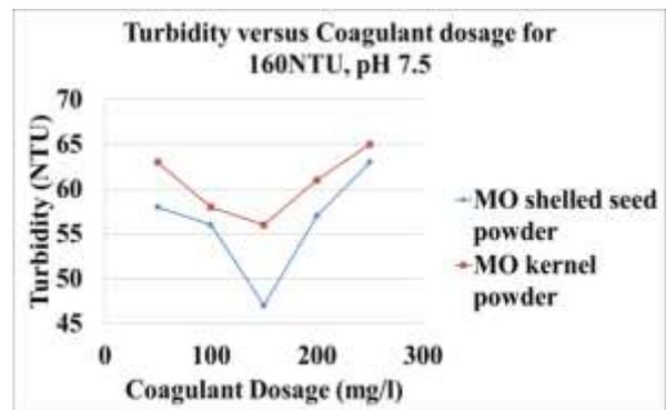
Fig 7: Residual turbidity v/s coagulant dosage
