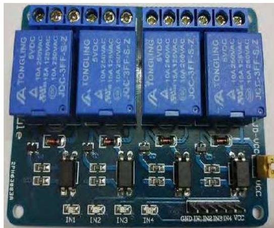
Figure 4: 4 Channel Relay Board
