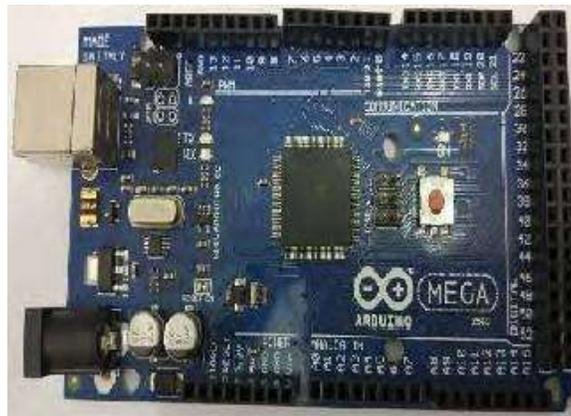
Figure 1 Arduino Mega 2560
