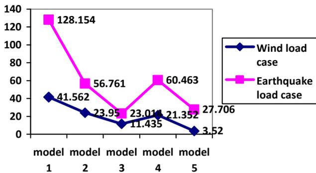
**Fig.3.3:** Variations of maximum Absolute Displacement in mm with different types of Model.
