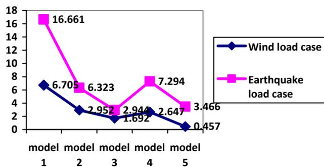
**Fig. 3.4:** Variations of maximum Storey Drift in mm with different types of Model.
