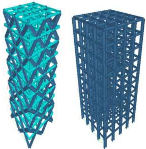
Model III – Steel diagrid with concrete frame. Model IV – Steel Bare Frame.
