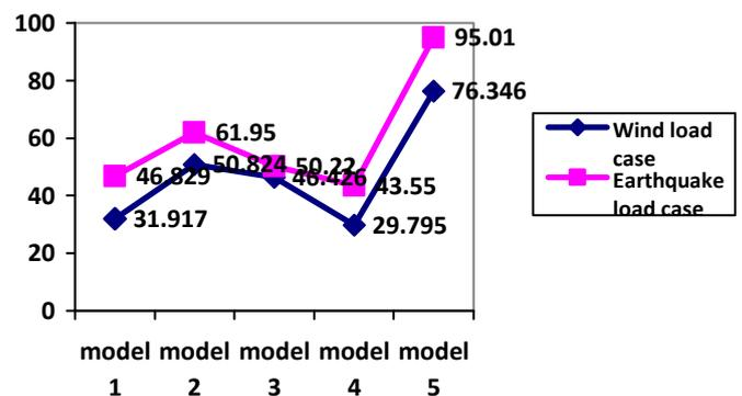
Fig. 3.2: Variations of maximum Shear Force in kN with different types of Model.
