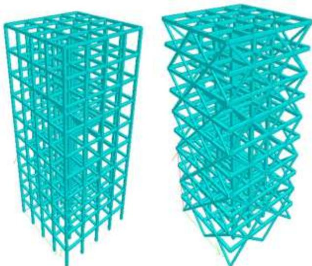
Model I – Concrete Bare Frame Model II – Concrete diagrid with concrete frame.
