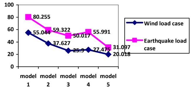
Fig. 3.1: Variations of Maximum Bending Moment in kN with different types of Model.
