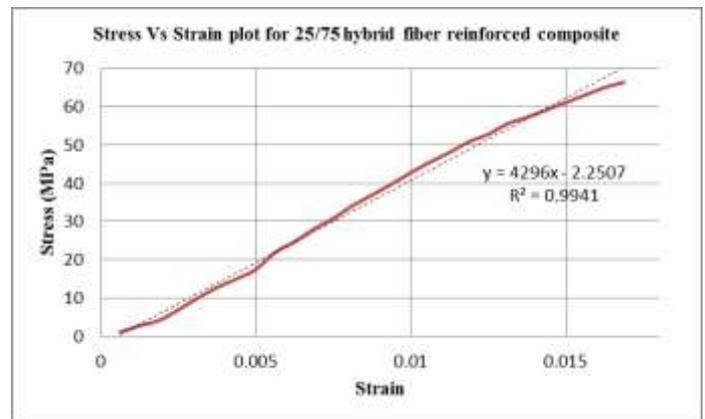
Fig 2.3: Stress-Strain Plot for Hybrid with 25/75 fiber distribution
