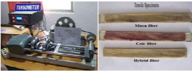
Figure 4.8: Tensometer and specimens
