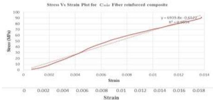
Fig 2.2: Stress-Strain Plot for Coir fiber reinforced composite
