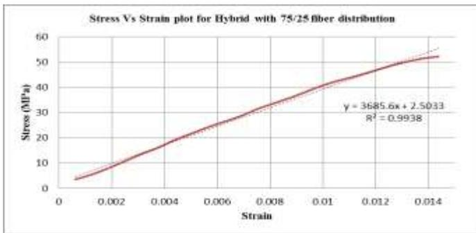
Fig 2.5 : Stress-Strain Plot for Hybrid with 75/25 fiber distribution
