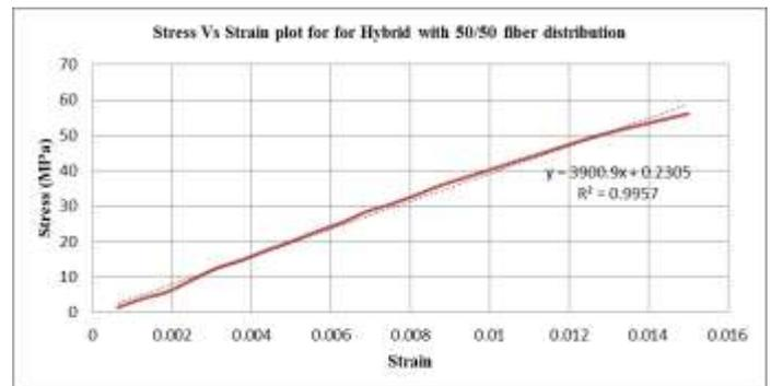
Fig 2.4: Stress-Strain Plot for Hybrid with 50/50 fiber distribution
