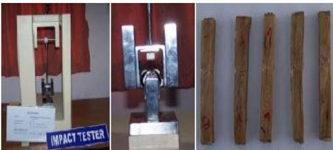
Figure 2.0: Impact test equipment, fixture and specimens
