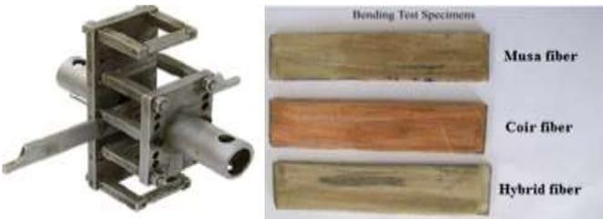
Figure 5.9: Bending test fixture and specimens
