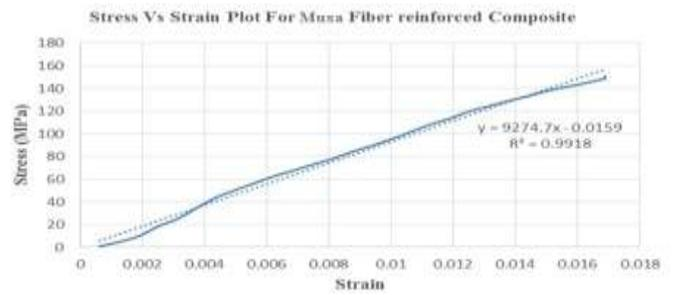
Fig 2.6: Stress-Strain Plot for Musa fiber reinforced composite
