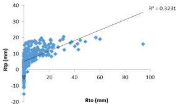
Fig 4.22 Correlation between observed and predicted rainfall by MLR-31, during the validation period.
