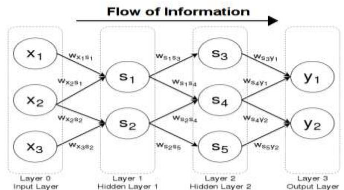
Fig 3.2 Four layer feed forward neural network
