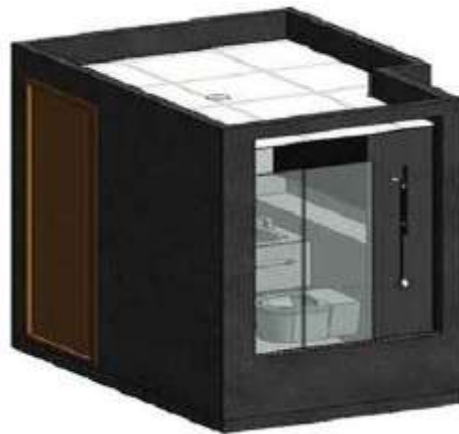
Fig -1.2: Diagrammatical representation of precast concrete volumetric PBU
