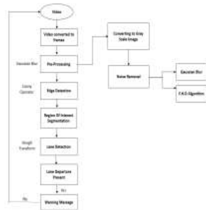
Figure (1) Lane Detection Flow Chart
