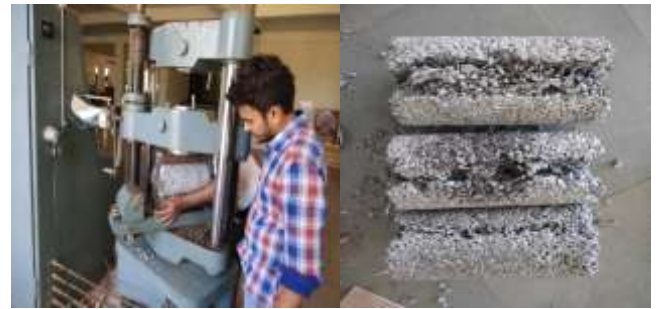
Fig. 4 Split tensile strength test
