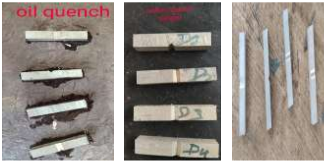
a) Oil quenched specimens b) Water quenched specimens vvvvvvvvvvc) Specimen cooled in atmospheric air
