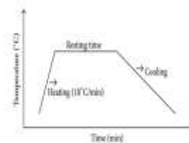
Fig. 5: Heat treatment cycle.
