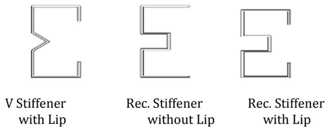
Fig-1: Typical view of channel sections
