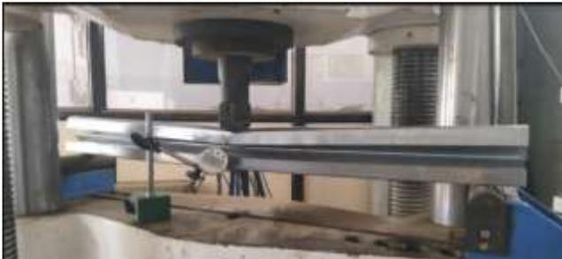
Fig-8: Channel section with stiffener failure pattern
