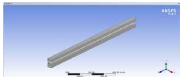
Fig-2: CFS section model
